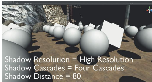
FIGURE 7.23 Settings that make the real-time shadows appropriate for this scene (they could all be different for a different scene with different lengths of visible distance).
